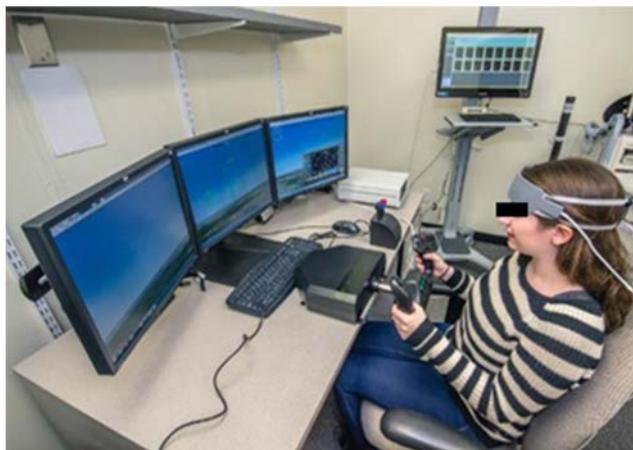
**FIGURE 3.2** Low-fidelity flight simulator with unmanned vehicle remote-piloting tasks while operator prefrontal brain activity is monitored with fNIRS.
