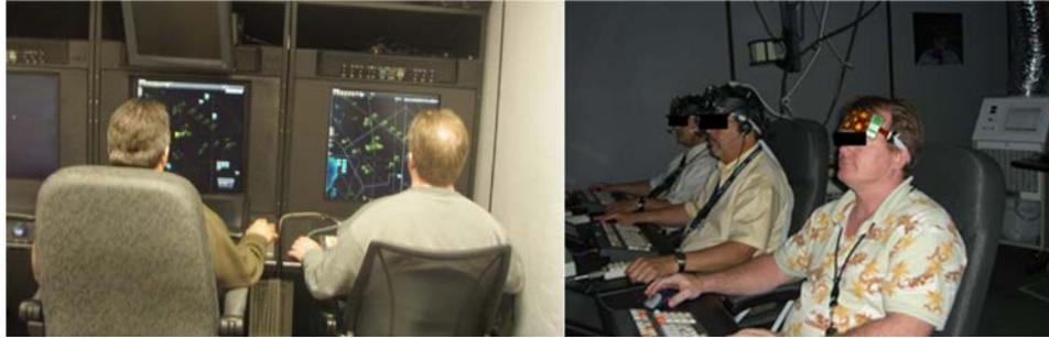
**FIGURE 3.1** Control workstations with high-resolution radarscope, keyboard, trackball, and direct keypad access (left). Operators in the study performing ATC tasks in front of workstations with a fNIRS sensor pad on their foreheads (right).
