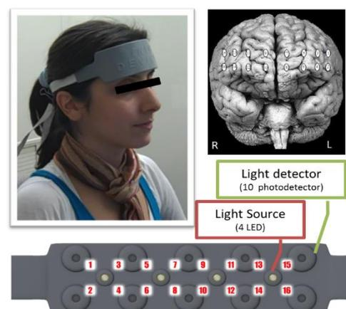
Figure 1: fNIRS sensor (top, left), projection of measurement locations (optodes) on brain surface image (top, right), optodes identified on fNIRS sensor (bottom).
